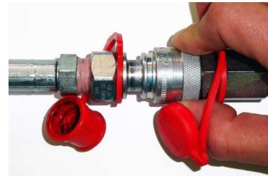
**ATTENTION:** the dust protection caps must put back on every time the hoses are decoupled.
