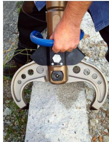
**ATTENTION:** When working be sure that only the tips are in contact with the concrete while the arms are not under load!
