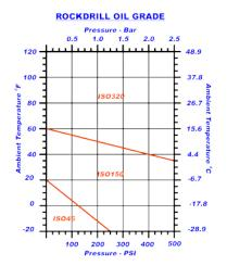
Remember: Insufficient lubrication or incorrect lubrication grades may result in damage being caused to the hammer and it's components. Hydraulic oils, engine oils, gear oils and diesel are not recommended for lubricating DTH hammers.
