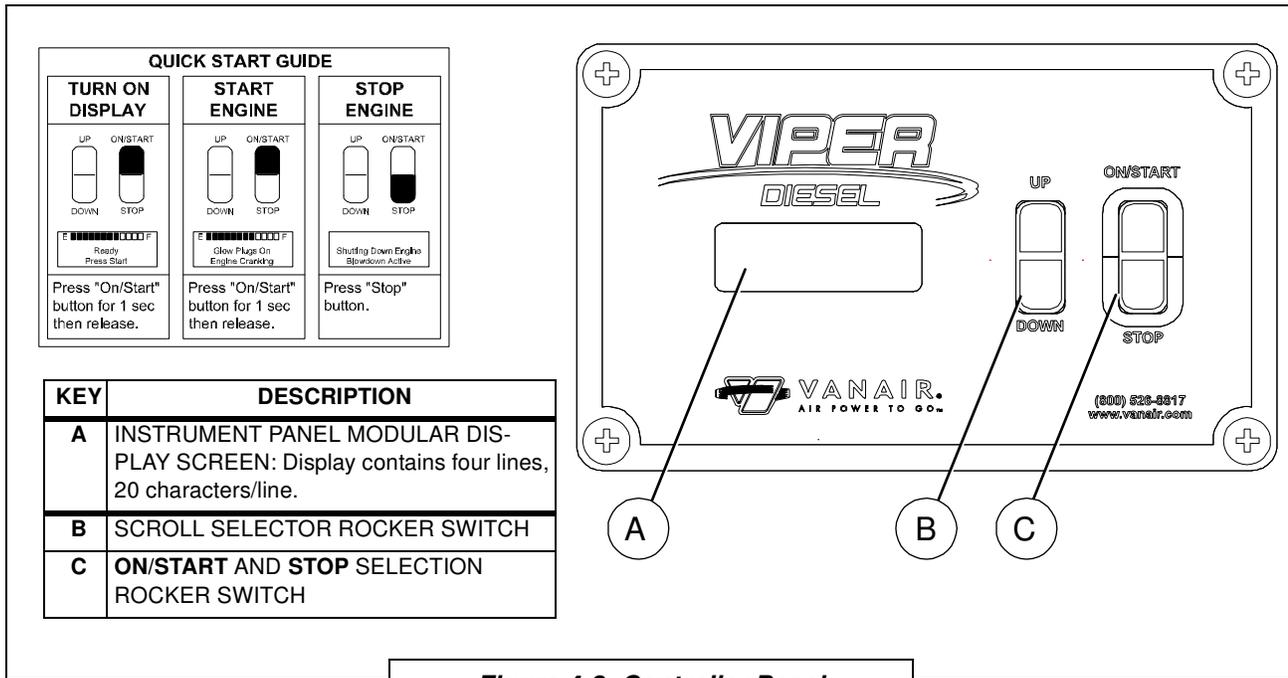
Figure 4-2: Controller Panel
