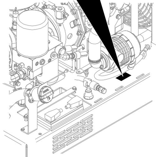
**Figure 6-1: Machine Serial Plate Location**
