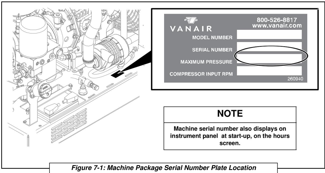
**Figure 7-1: Machine Package Serial Number Plate Location**
