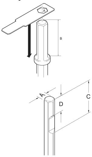
Use the gauge that corresponds to the insertion tool's shank dimension. See section "Technical data" for correct tool shank dimensions.
