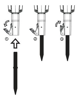
When fitting notched insertion tool, see the following steps:
