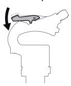
Start the machine by sqeezing the trigger while firmly holding the handle.
