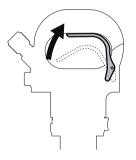
Start the machine by sqeezing the trigger while firmly holding the handle.
