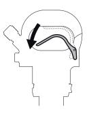
Stop the machine by releasing the trigger. The trigger returns automatically to the stop position.
