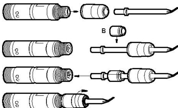
1. Slide the retainer over the shank and collar onto the chisel.
