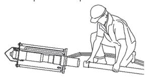
5. Lift the post and post driver to a vertical position. For long and heavy posts, two persons may be required.
