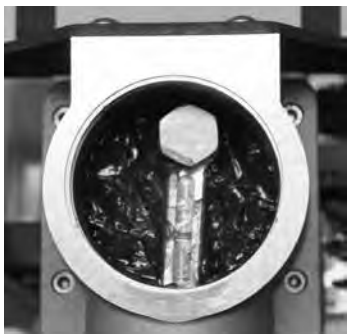
Fig. 10 - After completely cleaning out old grease, add new grease till level with the bottom edge of the crank pin head.
