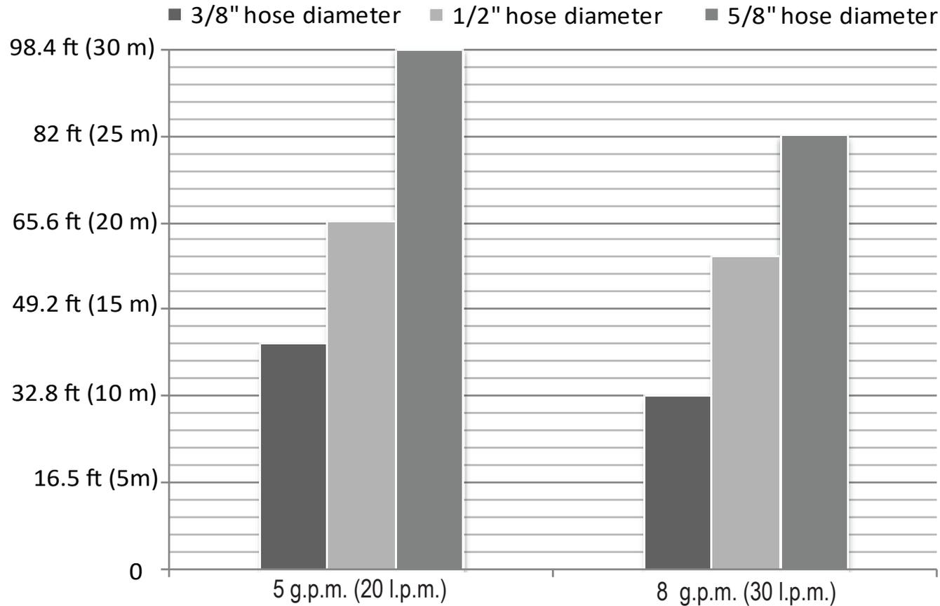
Pressure from power pack: 2200 psi (150 bar), Flow 5 g.p.m. (20 l.p.m.), zero elevation, 2 set couplings per 33 ft (10 m) hose.
